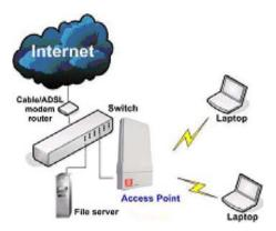
In the example above, the wireless users will be able to access the file server connected to the switch through the access point in **Access Point** mode.
