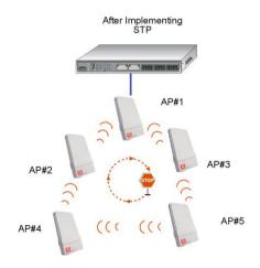
The path with the smallest cost will be used and extra redundant paths will be disabled.
