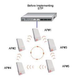
In short, the main purpose of activating STP is to prevent looping when you have redundant paths in the network. Without activating STP, redundant topology will cause broadcast storming.
