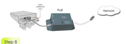
Connect the power adapter in the Compex PoE kit (not provided) to the main electrical supply and the power plug into the socket of the injector.
