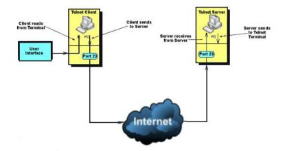
Telnet allows a computer to remotely connect to the NetPassage WPP54G CLI (Command Line Interface) for control and monitoring.
